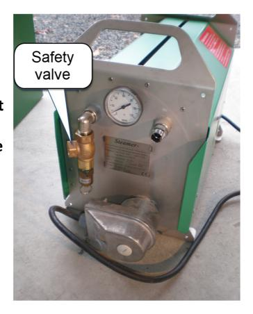
Always place the device on a surface that can withstand water, such as here on a concrete floor. If it is wood, linoleum or similar that cannot withstand water or can be damaged by heat, something must be placed under the
