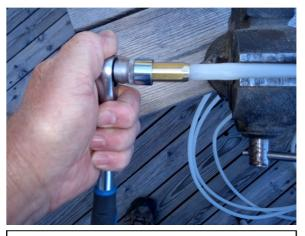
Align the nozzle and screw in onto the hose
